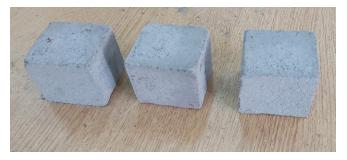
Figure 4: WPSA (25%) Mortar Samples.
