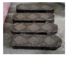
Figure 3: Mortar mix Casted in Moulds.
